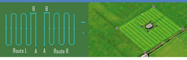
Using GROUND STATION, the user can select the operation area and set operation distance, flight speed, altitude, and other information.
